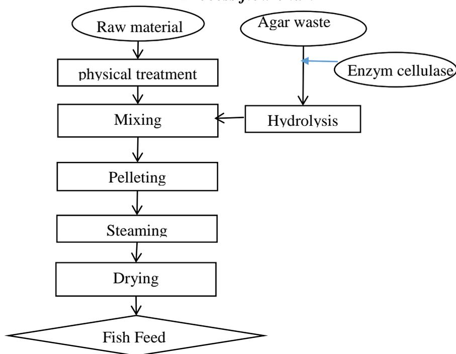
**Figure 3.19. Production processes for tilapia feed**
