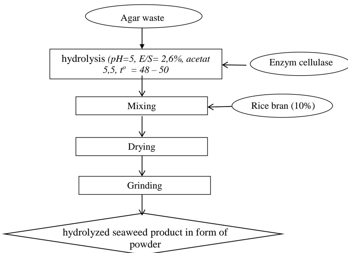
**Figure 3.18. Processes of hydrolysis of seaweed waste by cellulase from bacteria**
